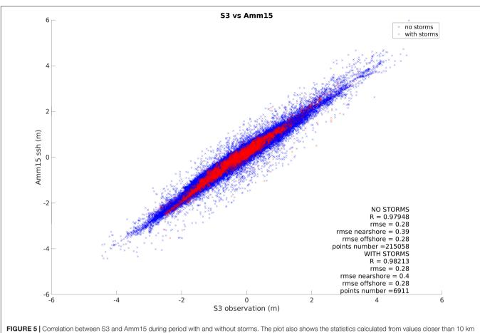
FIGURE 5 | Correlation between S3 and Amm15 during period with and without storms. The plot also shows the statistics calculated from values closer than 10 km from the coast (near shore) or further than 50 km from the coast (offshore).
