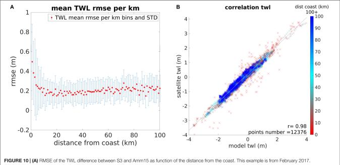
(B) Correlation between satellite and model data with color indicating distance to the coast from (blue) all data further than 100 km from the coast to (red) data at the coast. The RMSE in the right plot was averaged per kilometer bins.
