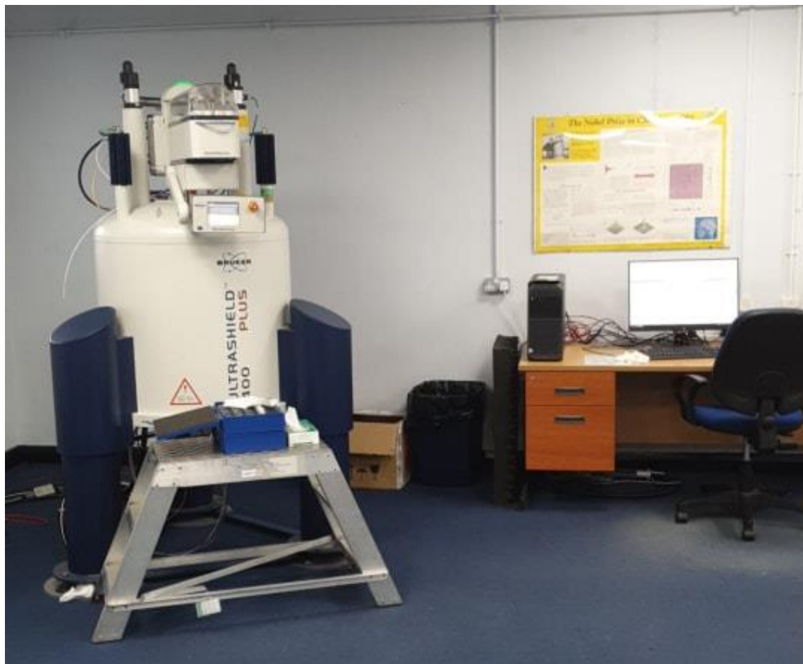
Image 2- 1: The Bruker 400 MHz Nuclear Magnetic Resonance machine used predominately throughout this project
