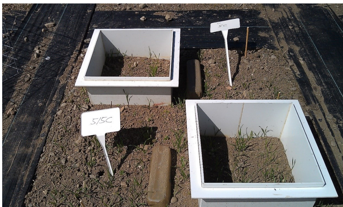
Fig 6.1. Two adjacent treatment plots, which had both received the same treatment in year 1, showing developing wheat plants, gas sampling chambers and \text{NH}_3 traps.
