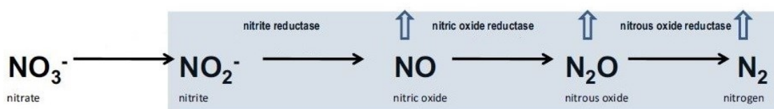
Fig 2.3. The denitrification process, showing the various products and catalysing enzymes. Adapted from Hirsch and Mauchline (2015).
