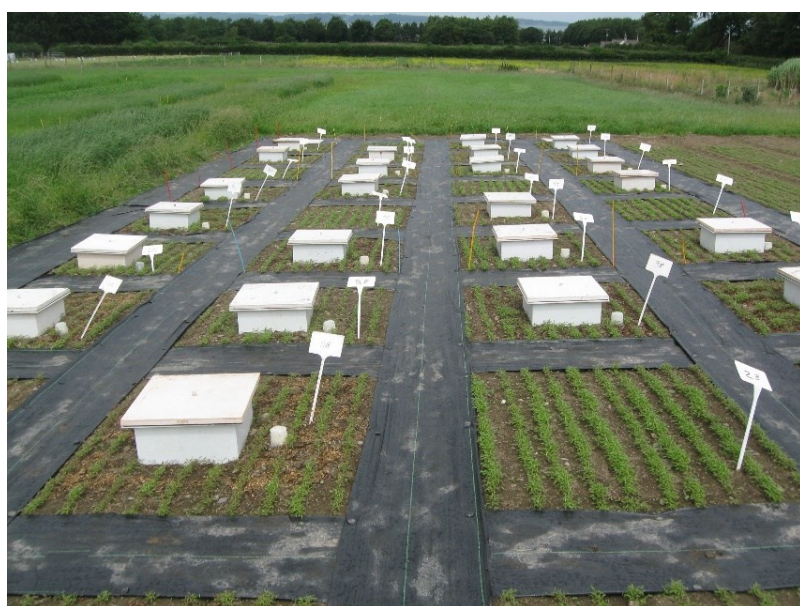
Fig. 5.1. Experimental area showing plots divided by buffer strips and fitted with gas sampling chambers.
