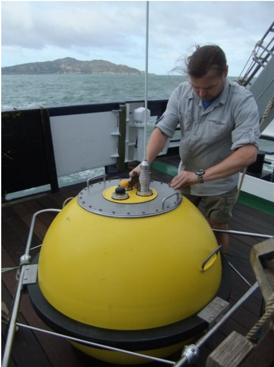
Figure 11.17: A Datawell Waverider surface following buoy ready for deployment to the west of Anglesey, Irish Sea, by Bangor University (Photograph: S. Ward)
