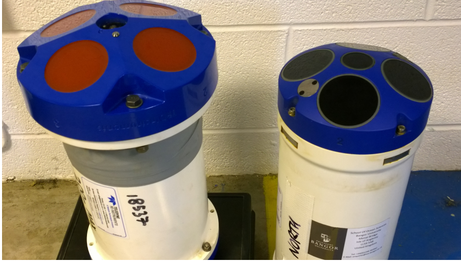
Figure 11.7: 4-beam (left) and 5-beam (right) acoustic Doppler current profilers (ADCPs).
