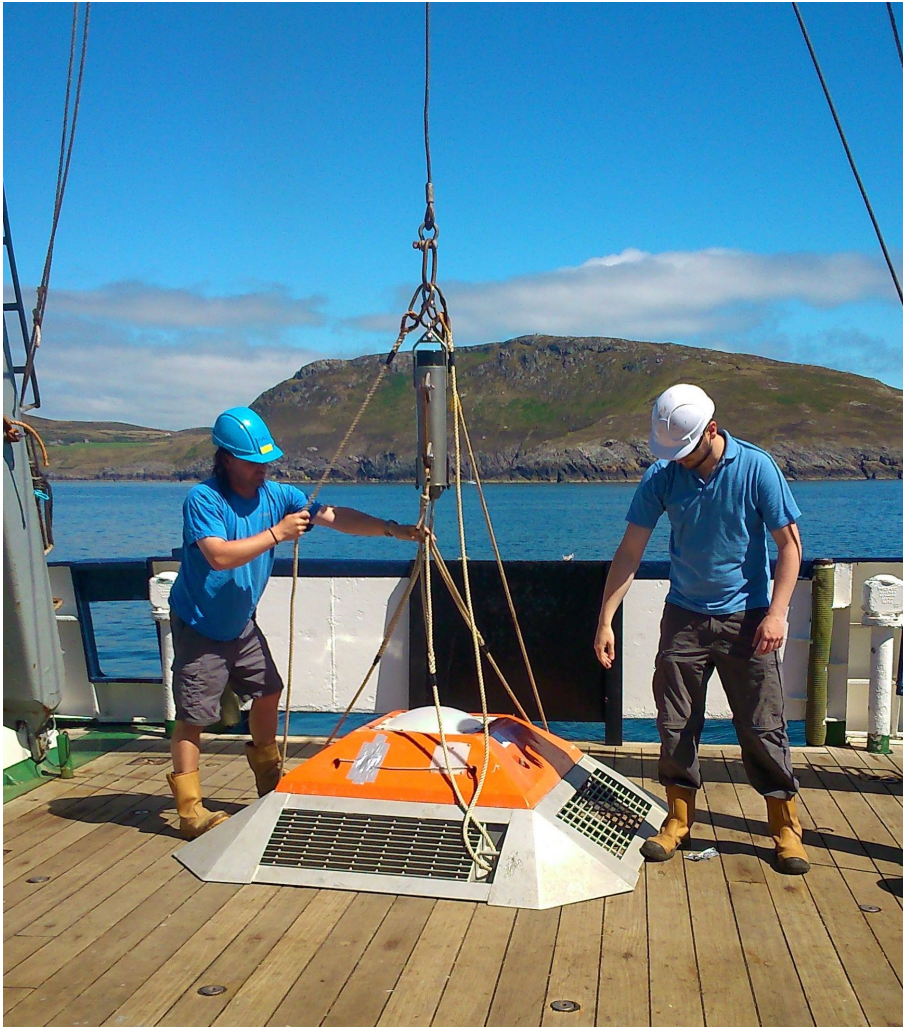
Figure 11.10: Low profile ('trawl-resistant') ADCP mooring. The acoustic release above the instrument is used during the deployment stage; a similar acoustic release, in the base of the instrument frame, is used during recovery. The orange part of the instrument, which is buoyant, separates from the heavy base when the (recovery) acoustic release is triggered. The top and bottom parts of the mooring are connected by a cable, which is coiled inside the base prior to deployment.
