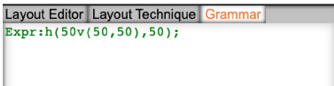
Figure 7.8: Shorthand grammar viewer. Users can write the shorthand grammar in this window, which will display (when updated) in other views. Using the shorthand users can create complex views, using some simple commands.
