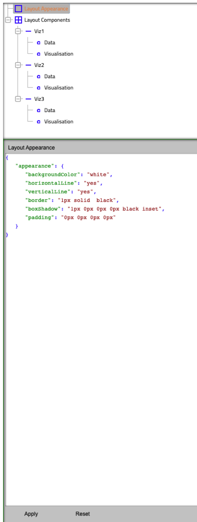
Figure 7.9: Layout Appearance views. The user can adapt different aspects of the appearance. They are able to choose a specific Component of the layout. The tree is automatically updated from the information in the MVG grammar. Subsequently, users can then select the Viz, add the Data and the Visualisation code. Here the Layout appearance is shown in the lower view. Users can change the parameters to adapt how the views appear.
