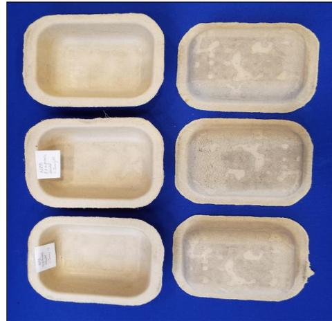
Figure 3. Punnets made from atmospherically refined EFB fibre
