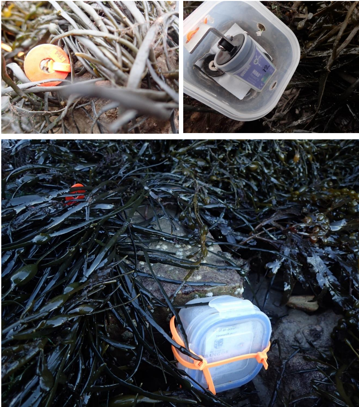
Figure 4.3. Loose intertidal rocks were marked with coloured, labelled, washers. Onset HOB0 Pendant G loggers (UA-004-64) were placed in a plastic housing on selected rocks to measure their movement (acceleration and change in inclination).
