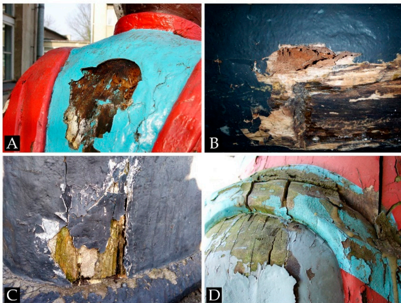
Figure 4. Damage of wooden objects covered with paints ((A–D): artefacts from the collection of The Museum of Apiculture in Swarzędz, a branch of The National Museum of Agriculture and Food Industry in Szreniawa, Poland).
