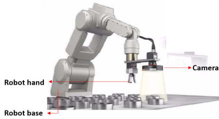
FIGURE 1. Vision guided robot for pick-and-place application [19].
