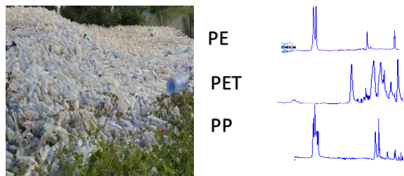
Fig. 5.3 Diagram showing the identification of polymeric materials by FT-IR (Author's image)
