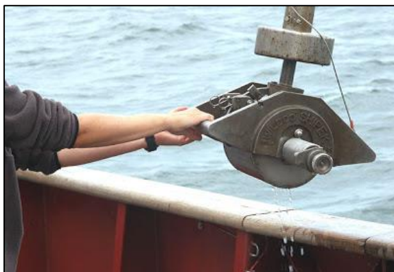
Figure 2.2: Wildco 860-A10 grab sampler when retrieved with sediment. (source: http://attleborobio.blogspot.com/ ).
