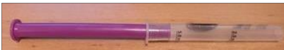
Figure 2.9: Syringe used for down-core sampling of the sediment bed in the flume
