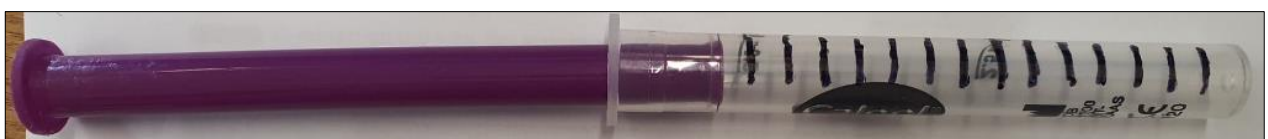
Figure 4.11: Syringe, sub-divided every 5 mm used for the laboratory sediment 'core' sampling.
