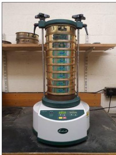
Figure 2.6: Endecott's Octagon 200 vibratory sieving machine used for PSA of sediment samples.
