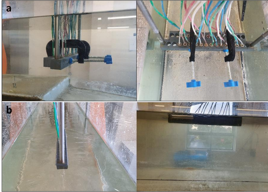
Figure 2.8: Array of 24 transducers used for perpendicular to the flow scans (a) and array of 16 transducers used for parallel to the flow scans to record bedform development and migration rates during the laboratory experiments (b).
