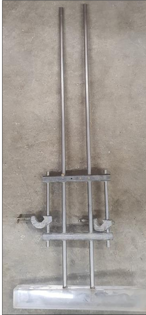
Figure 4.3: PVC block used for sedimentary bed flattening when setting up the flume for the laboratory experiments.
