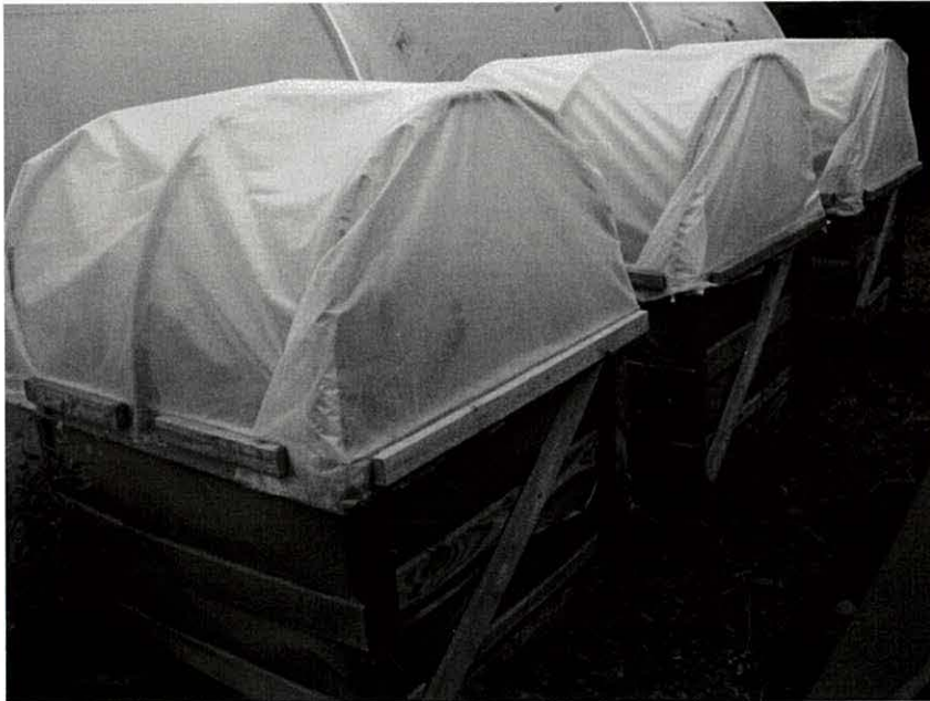
Plate 3 Hoods positioned on artificial slate waste tips at Penrhyn Quarry to exclude all atmospheric precipitation
