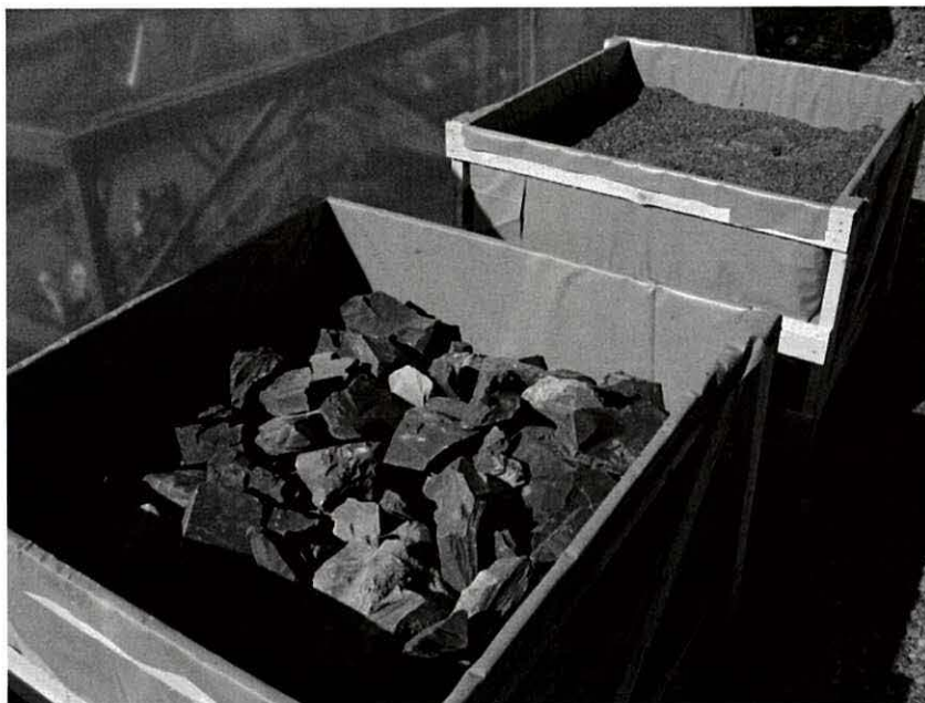
Plate 1 Artificial slate waste tips at Penrhyn Quarry, part way through filling with large fraction pieces of slate waste (left box) and addition of slate sand (right box)
