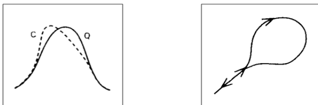
Figure 1.14 – Single valued line and loop where concentrations ( C ) and discharge are uncoincidental. The loop on the higher discharges means that levels of metals and discharge do not coincide in the middle of the hydrograph (Williams, 1989).
