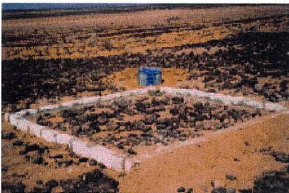
Figure 3.11: Runoff plot experiment at Marab Hassan .
