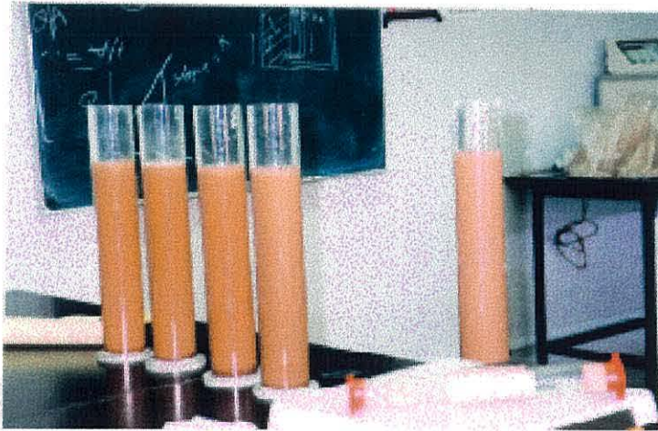
Figure 3.3: Bouyococ Hydrometer method for measuring soil texture.
