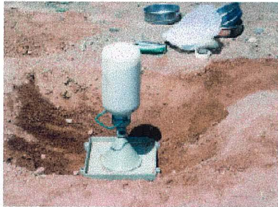
Figure 3.8: Ottawa sand cone test for measuring soil bulk density in Marab Hassan.
