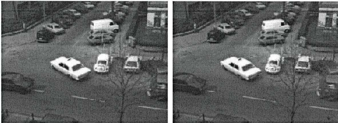
Figure 4.4: Images 3 and 4 of the Taxi set of images used for testing optical flow systems
