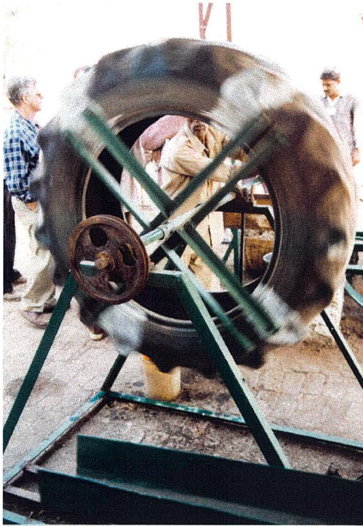
Plate 3.8 Hand-operated grass seed pelleting machine promoted by IGFRI used to make grass pellets for broadcasting in the project area (1997).
