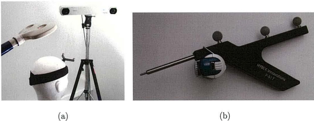
Figure 4.3: The tools being tracked: (a) The subjects head, The electromagnetic coil and (b) the viewpoint of the operator captured using a webcam aligned with the digitizing probe
