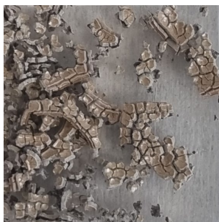
Figure 124. \text{ZrO}_2 produced from oxidising Zircaloy-2.
