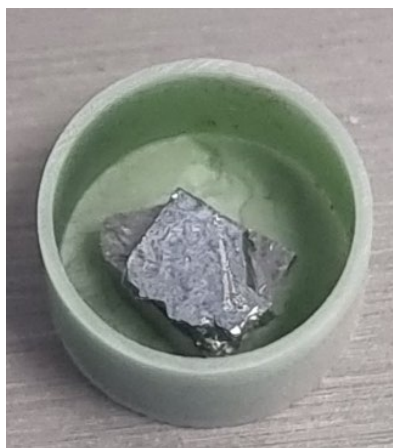
Figure 109. Zr and Cr after heating in Ar to 1500^\circ\text{C} . Discolouration of the \text{Y}_2\text{O}_3 crucible can be observed compared to Figure 105 .
