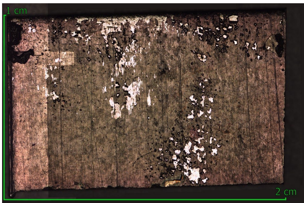
Figure 100. Optical microscope image of Cr-MoNbTaW sputtered onto Zircaloy-2 cladding material. 59 images were taken and manually stitched together in the Inkscape software. Light grey: Zr; brown: Cr.
