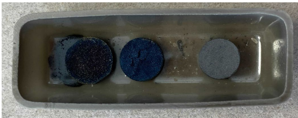
Figure 84. Pellets of equiatomic MoNbTaTiW after sintering for a dwell time of 6 hours, and according to the conditions in Table 12 . From left to right: pellets 1 – 3.
