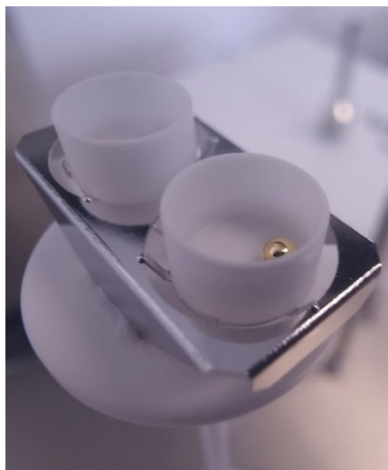
Figure 105. Au wire heated to 1200 in Ar in a \text{Y}_2\text{O}_3 crucible.
