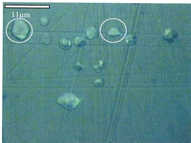
Fig 7.13 Optical micrograph showing growth of cadmium nuclei on a 6 \mu\text{m} textured glass substrate.
