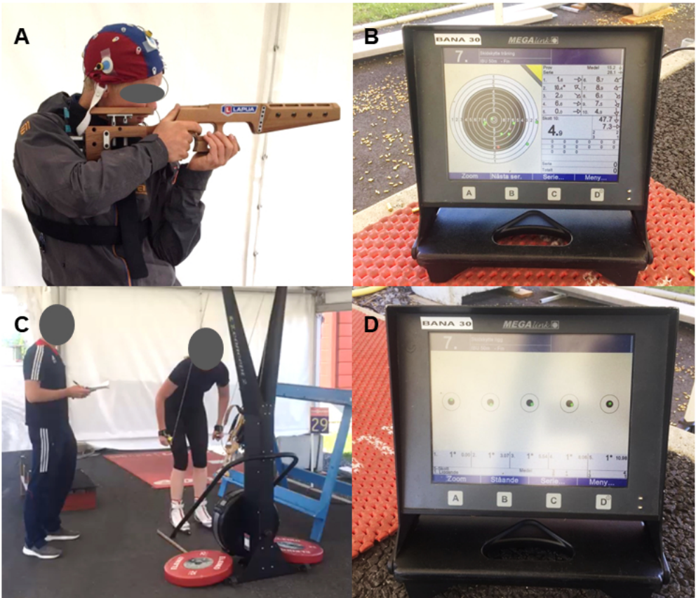
Figure 1. Illustrations of the field-testing setup for (A) an athlete equipped with the EEG electrodes and nylon cap during the standing phase of the precision shooting test (a dummy rifle is pictured here); (B) the target system used for the shooting precision test; (C) an athlete demonstrating double poling on the ski ergometer used for the simulated performance test; (D) the “hit or miss” target system used during the shooting phase of the simulated performance test.
