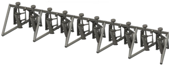
Figure 2.9: Repetitive Energy's 100 kW HEC River Array, comprising an array of Smart Stream turbines.
