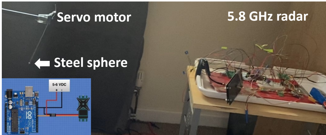
Figure 3.33: Steel sphere moving in a pendulum setup placed in front of the 5.8 GHz V1 radar. Inset shows the Arduino and stepper motor connection.
