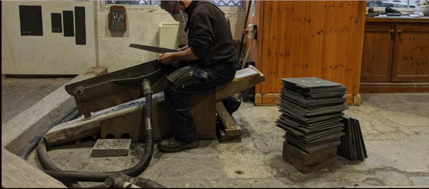
A demonstration of a quarryman splitting slate at the National Slate Museum. Photographed at the National Slate Museum in Llanberis, north Wales.
