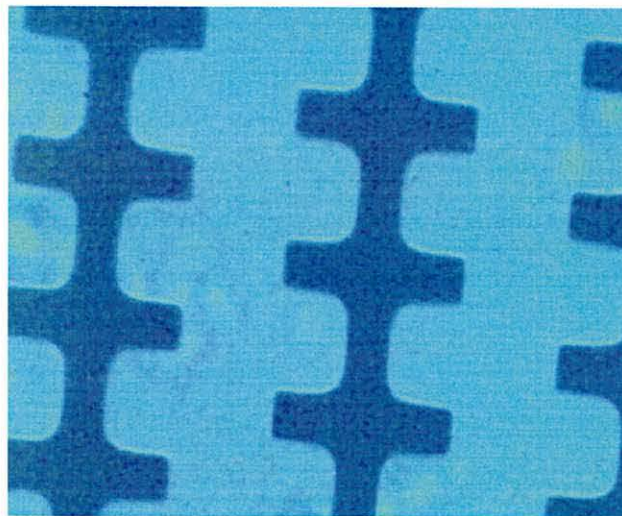
Figure 7.5 Image of the electrode structure shown in Figure 6.8 produced using a reversed low cost camera lens as shown in figure 7.4B
