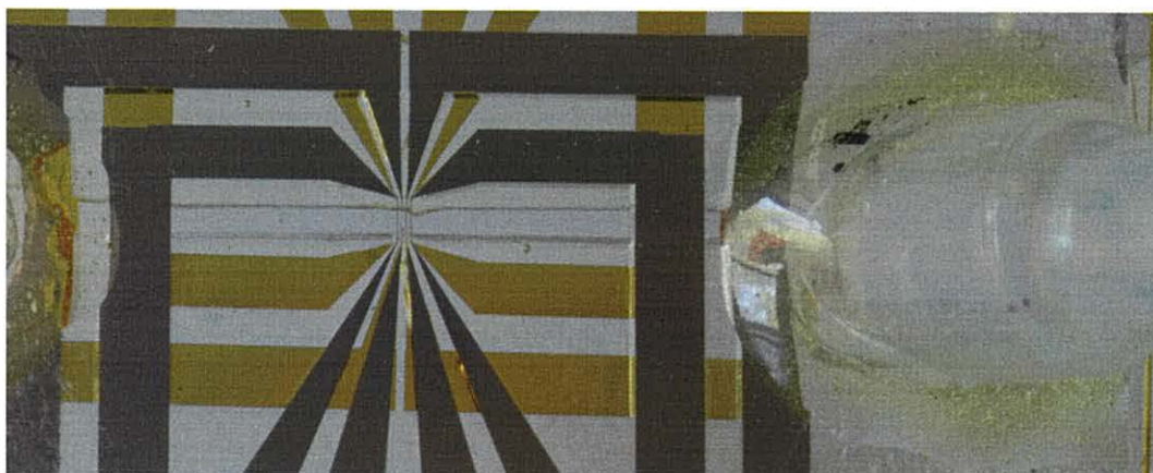
Figure 4.38 Channel structure produced using UV curing adhesive.
