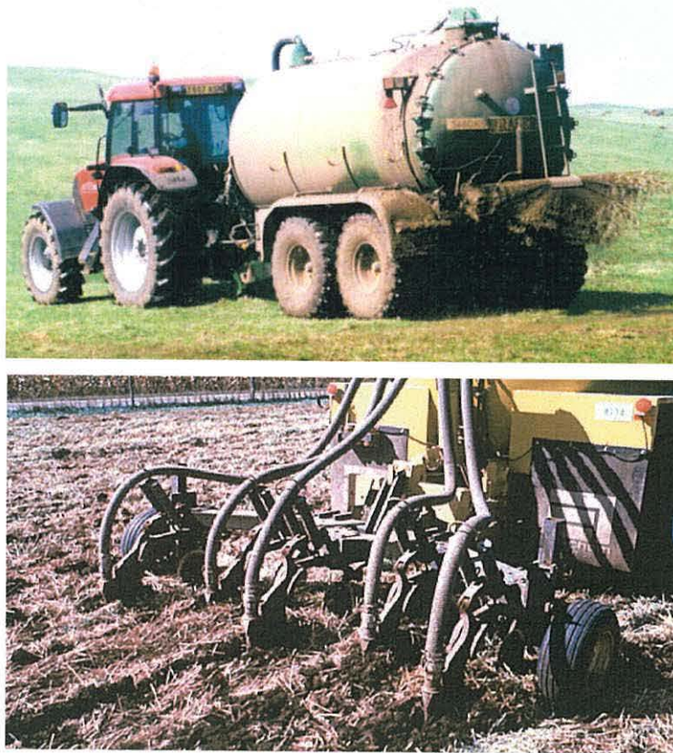
Figure 2.21. Conventional surface spreading (top) and contemporary deep-injection (bottom) of slurry.
