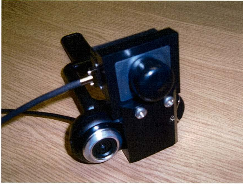
Figure 3.7: The application bracket with the VisTracker and webcam in place
