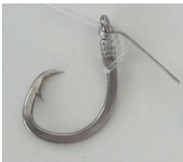
Figure 4. Circle hook modified with a wire appendage.
