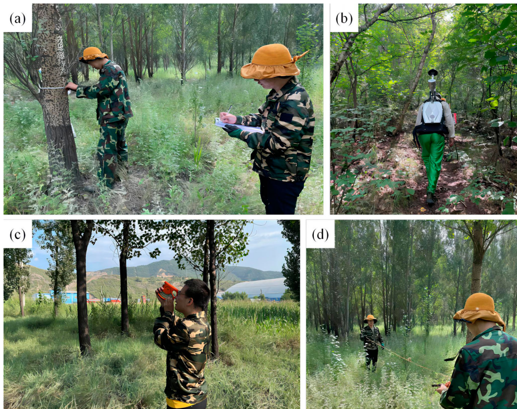
Figure 2. Forest sample plot survey (a) single tree diameter at breast height measurement using a diameter at breast height ruler; (b) scanning the forest sample plot using a backpack LiDAR; (c) single tree height measurement using a height gauge; (d) measuring the extent of the forest sample plot using a measuring rope.
