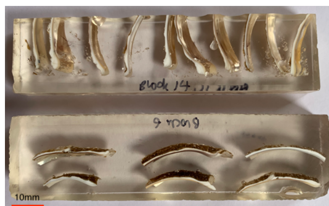
Figure 2.8: Fine polished blocks of Buccinum undatum shells embedded in resin. Cross sections allow internal shell layers to be visible under Raman microscopy.
