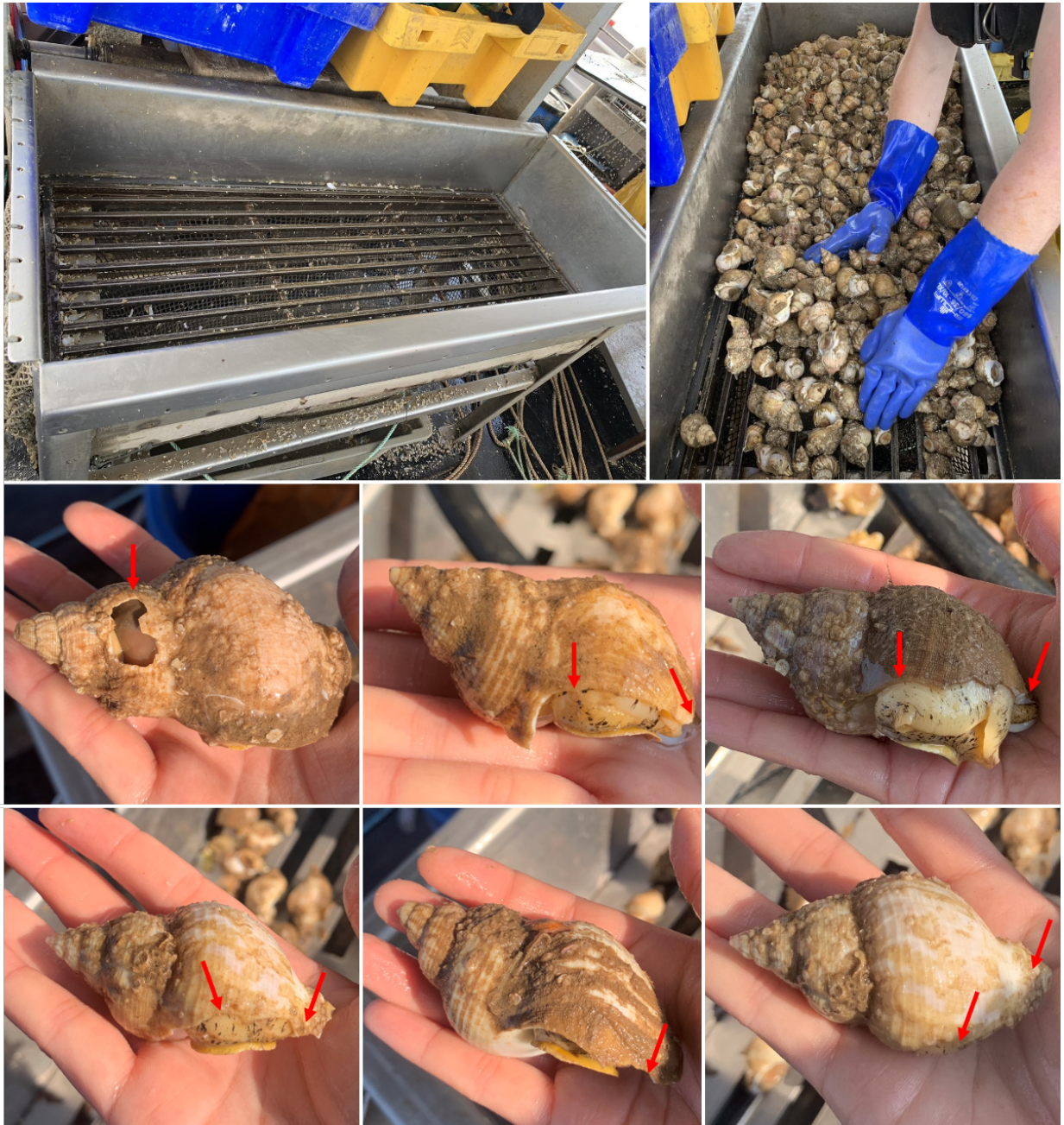
Figure A1. 4: Flat riddle on board commercial whelk fishing boat. Red arrows show areas of shell damage from the riddling process.
