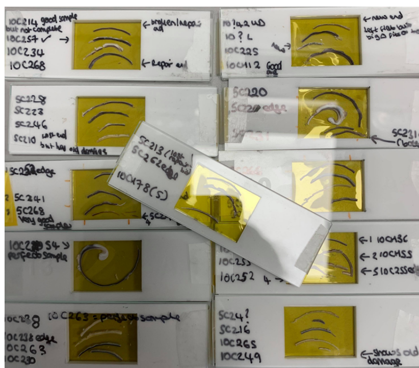
Figure 4.8: Thin shell sections of Buccinum undatum adhered to Kapton tape on custom microscope slides for \mu XRD analysis.
