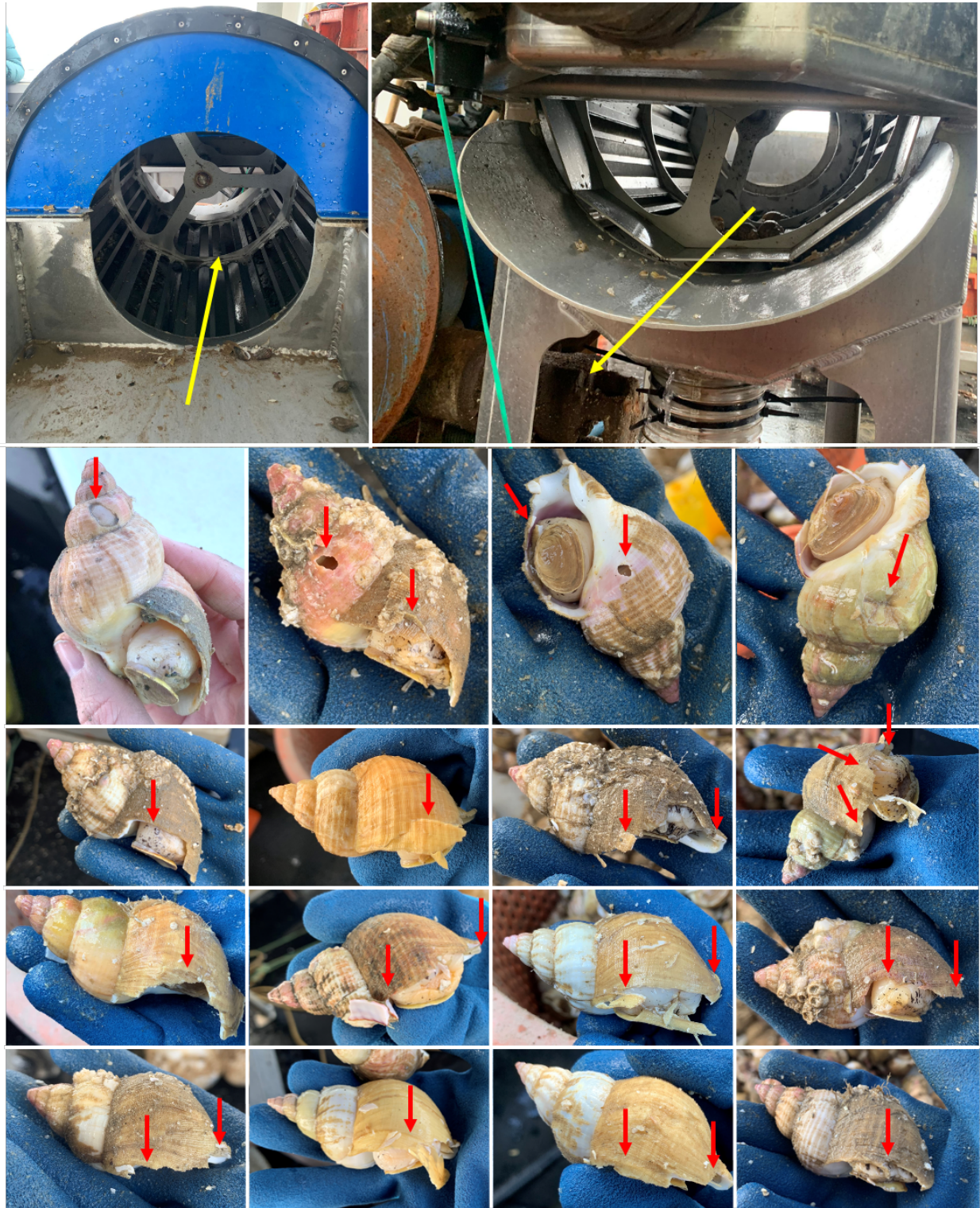
Figure A1. 3: Rotary riddle on board commercial whelk fishing boat. Yellow arrows indicate direction of whelk travelling through the metal frame. Red arrows show areas of shell damage from the riddling process.
