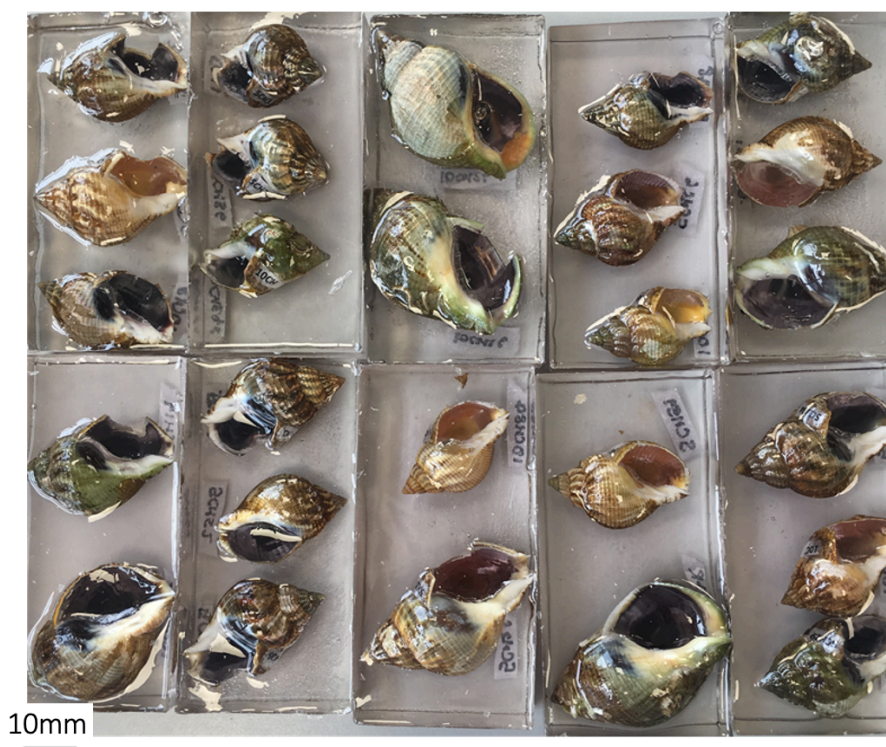
Figure 4.5: Cured and hardened resin blocks containing whole Buccinum undatum ready for thin section preparation.
