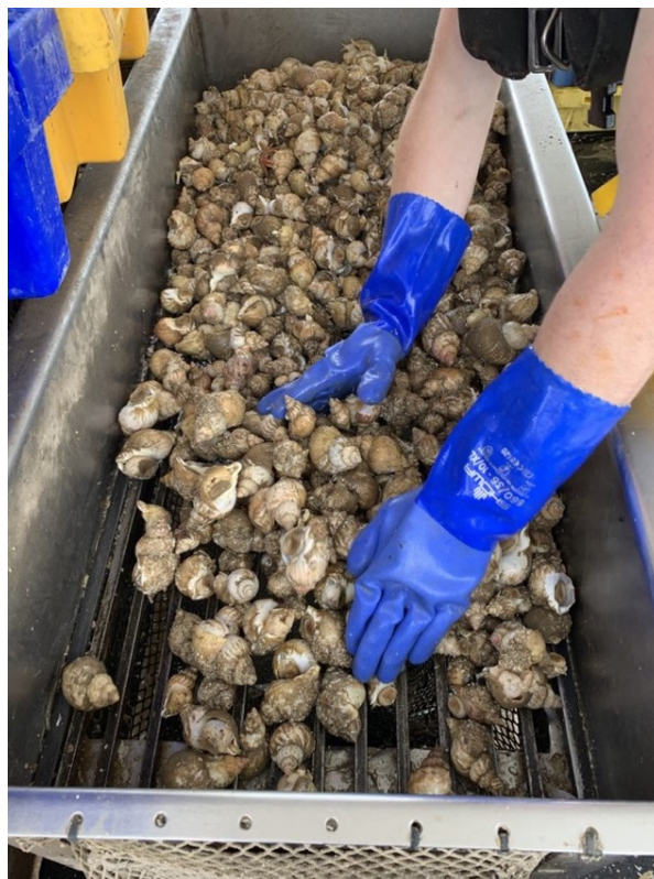
Figure 1.7: Commercial whelk riddle used to filter whelk samples to collect those above the minimum landing size (UK 45 mm).
