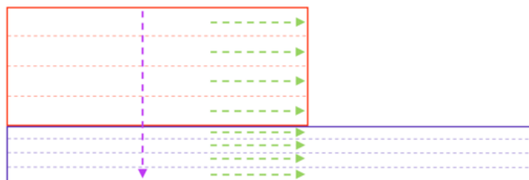
Figure 5.4: Diagrammatic representation of the whelk shell (red) with new growth (purple) and transects marked for ablation. Shell layers marked with dashed lines, purple arrow direction from outer to inner shell layers used for vertical laser traces and green arrows the laser ablation tracks horizontally within individual shell layers.
