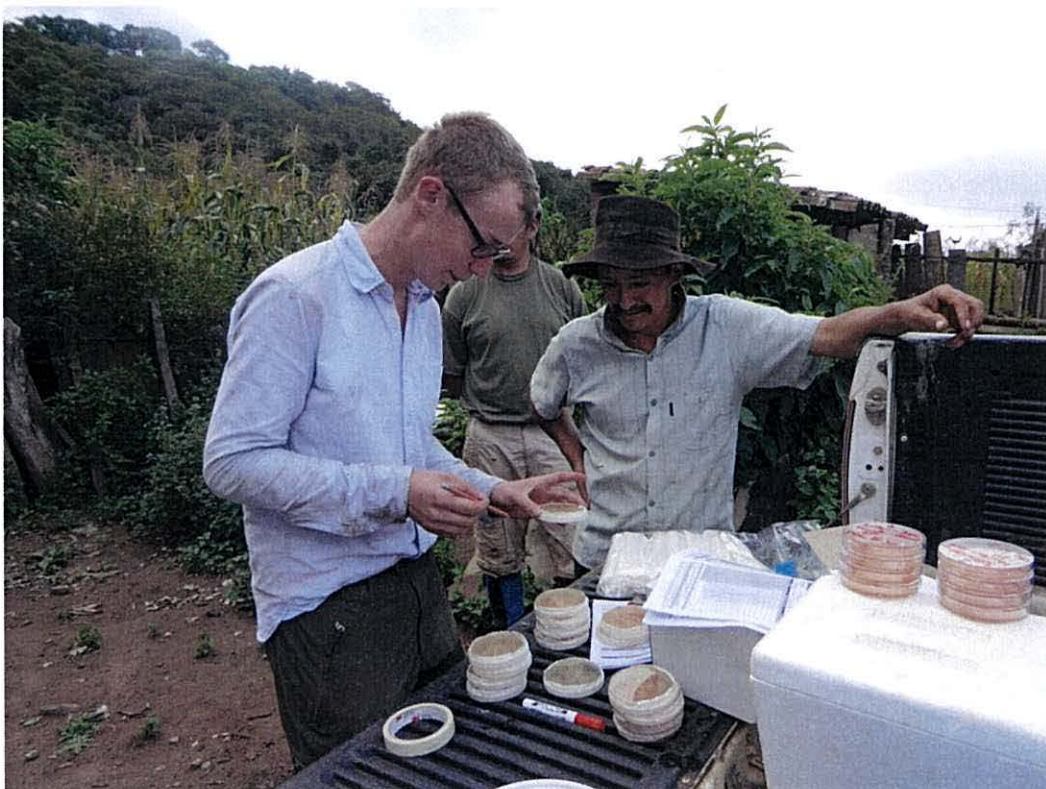
Figure E.2. Plating out and enumeration of E. coli and other coliforms in the field.
