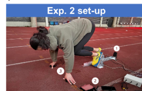
Figure 2. Sprint starting block set-up. 1-auditory stimulus, 2-visual stimulus, 3-haptic stimuli.
