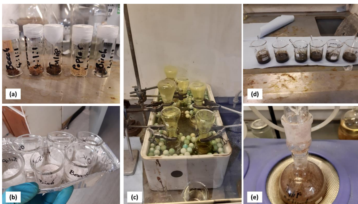
Figure 3-4 Sample preparation for the isolation of wood polymers, (a) wood solvent extractives after rotary evaporation, (b) \alpha -cellulose in sinter crucible, (c) holocellulose preparation with NaClO 2 in hot water bath, (d) Klason lignin preparation in 72% sulphuric acid, (e) Klason lignin preparation under reflux.
