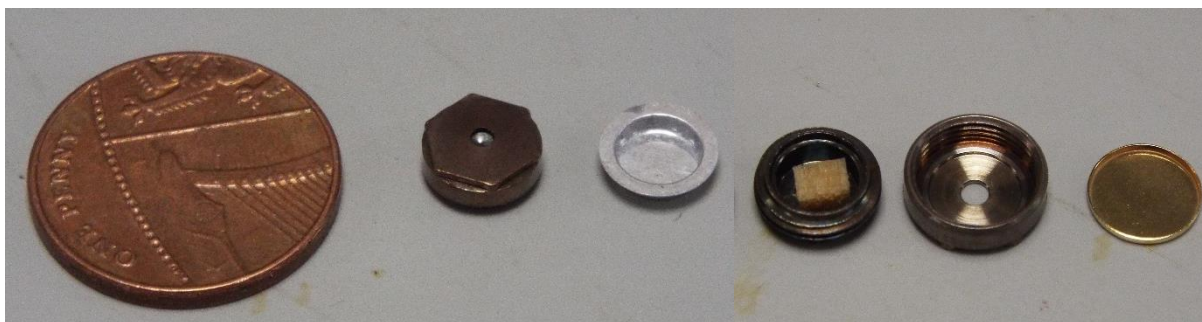
Figure 4-4 (left) High-pressure crucible and open crucible next to a one penny coin for scale. (right) Wood section inside the pressurised crucible before it is sealed.
