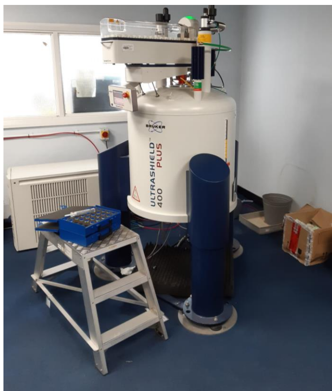
Figure 3-5 Bruker 400 MHz Ultrashield+ NMR spectrometer used for solution-state NMR studies in this thesis.
