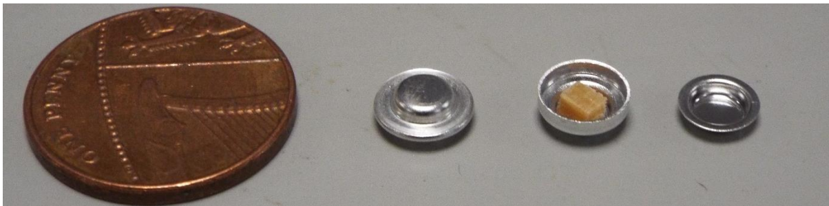
Figure 8-1 DSC crucibles used for thermoporosimetry next to a one penny coin. Water-soaked solid wood samples were sealed in the crucible using sealing tool.
