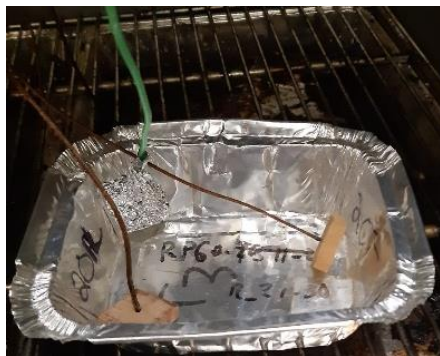
Appendix 40 (left) Thermocouples and wood samples used for the temperature measurement. (right) Temperature profiles during heat curing are similar for Wood A and B, despite slightly different moisture contents prior to cure.
