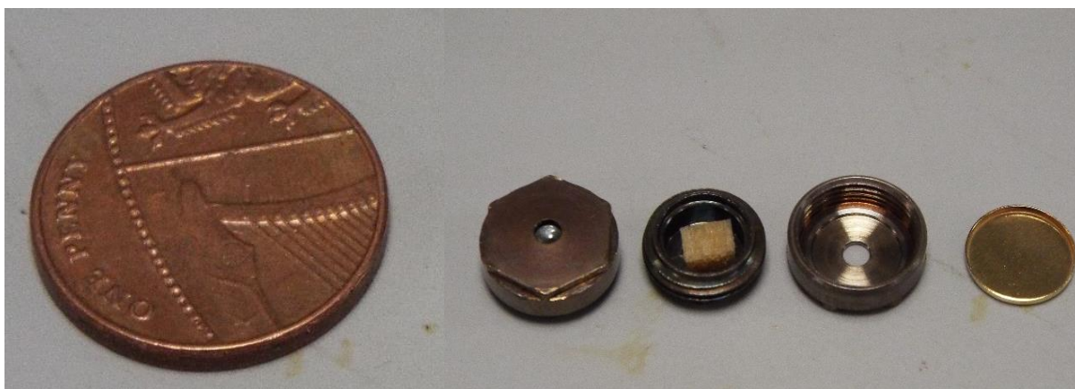
Figure 7-1 High-pressure crucible next to a one penny coin and wood section inside the pressurised crucible before it is sealed.
