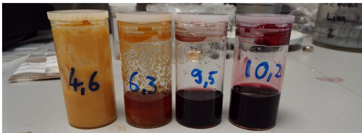
Figure 4-3 The colour of the studied PUF resin changes with the pH value. PUF resin adjusted to different pH values by adding either acetic acid (99% w/w) or potassium hydroxide pellets. From left to right: pH 4.68, pH 6.3, pH 9.5 (default), pH 10.26.
