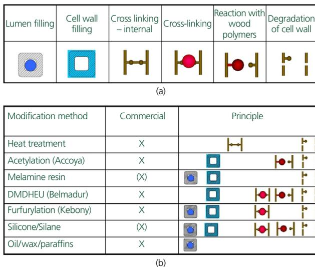
**Figure 1.** (a) Diagrams illustrating five types of wood modification which occur at a cellular level. (b) Summary of the combinations of modification process which occur together in each of the main wood modification technologies (adapted from Militz (2007))
