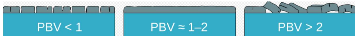
Figure 14 Visualisation of the Pilling Bedworth ratio. To the left, a ratio less than one. The middle is between 1 and 2 and the right has a ratio greater than 2 [2].
