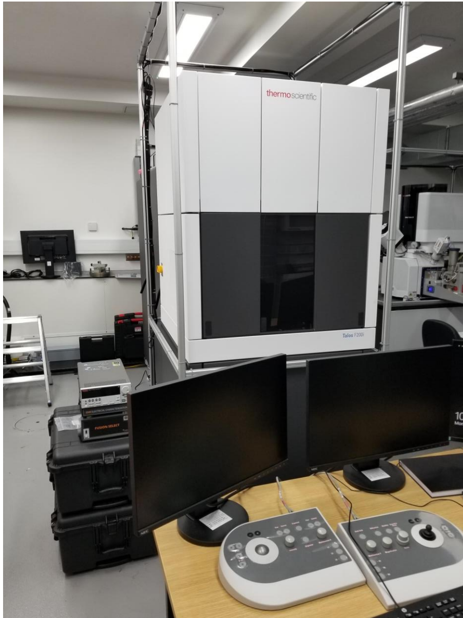
Figure 106 STEM with EELS equipment at the department of materials, Imperial College London.
