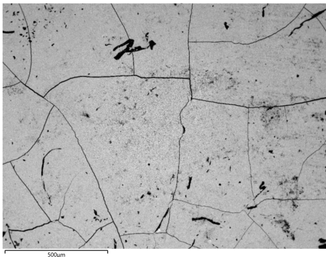
Figure 99 Pure amorphous \text{ZrO}_2 pellet pressed and viewed through SEM (12000 x magnification)
