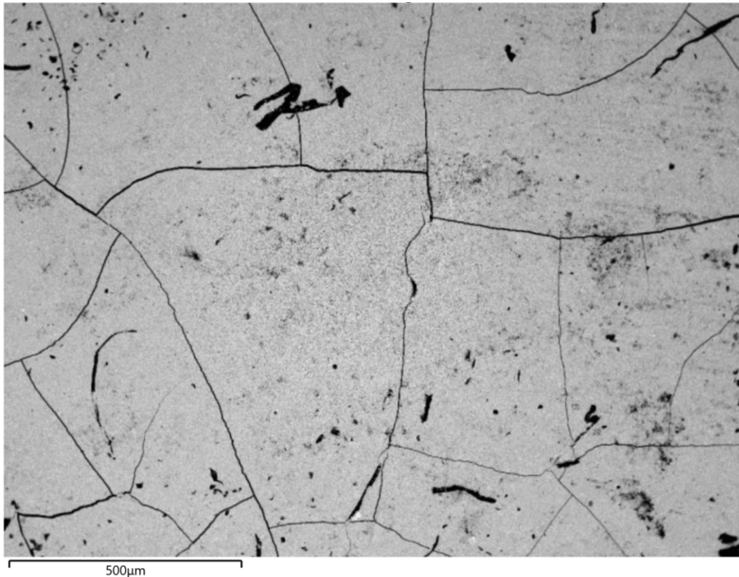
Figure 99 Pure amorphous ZrO 2 pellet pressed and viewed through SEM (12000 x magnification)
