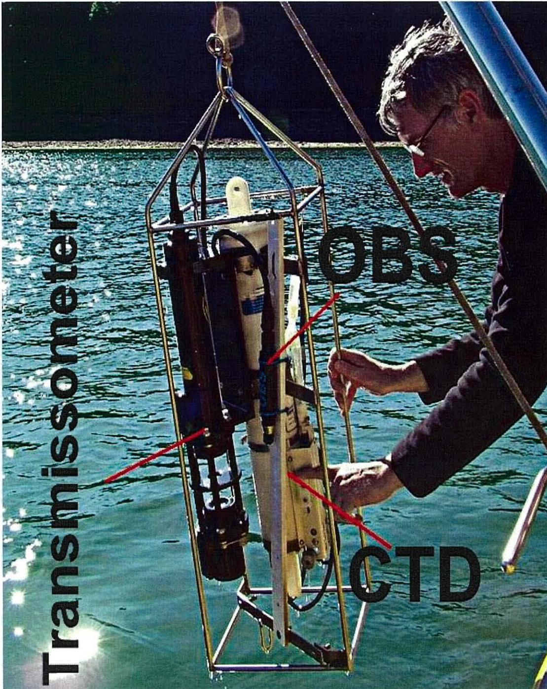
Figure 3.1 Photograph provided by Ben Powell and it shows the CTD, OBS and the transmissometer units on the frame, during a survey.
