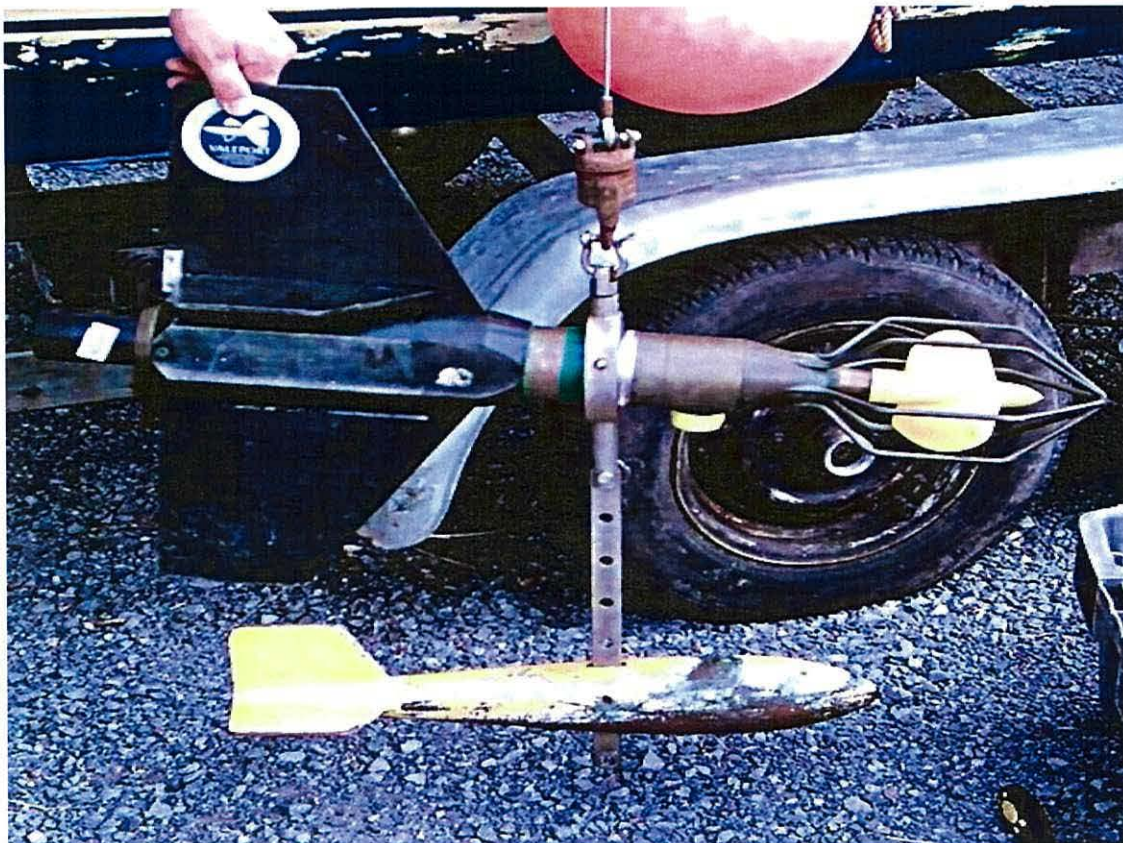
Figure 3.3 Photograph provided by Ben Powell and it shows the Valeport current meter, during a survey.
