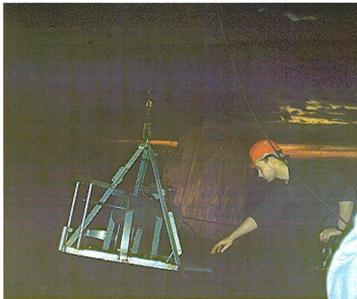
Photograph 2 Instrumentation used in the survey of offshore sites in the Humber estuary and along the East coast. Showing the Par-tec100 mounted in a heavy duty tripod with stabilising fin.
