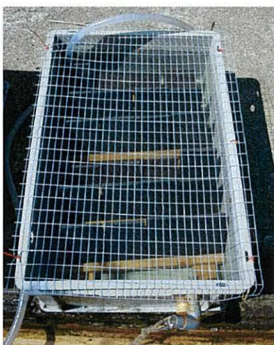
Figure 2 a-c. a) Diagrams showing the procedure used for the biofilming of experimental surfaces: slate tiles and assay slates and glass microscope slides. b) Tanks with running seawater used for biofilming of slates outside laboratory; two tanks were fed constantly with running seawater, the other (middle tank) was drained for 3-4 hours daily. c) slates held in grooved wooden racks within tank. Seawater (gravity fed from the laboratory system at 2 l/min) was fed into the bottom of the tank at one end and drained from the other end.
