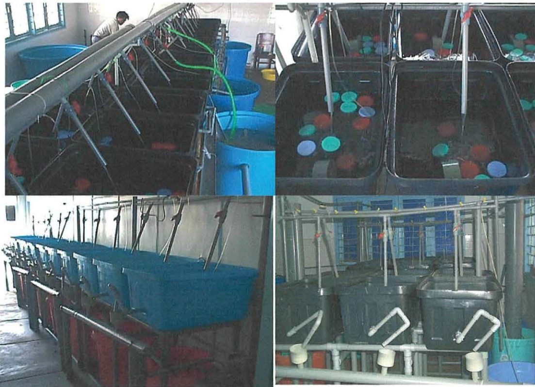
Figure 2: The recirculation system used for salinity experiments carried out in Can Tho laboratory.
