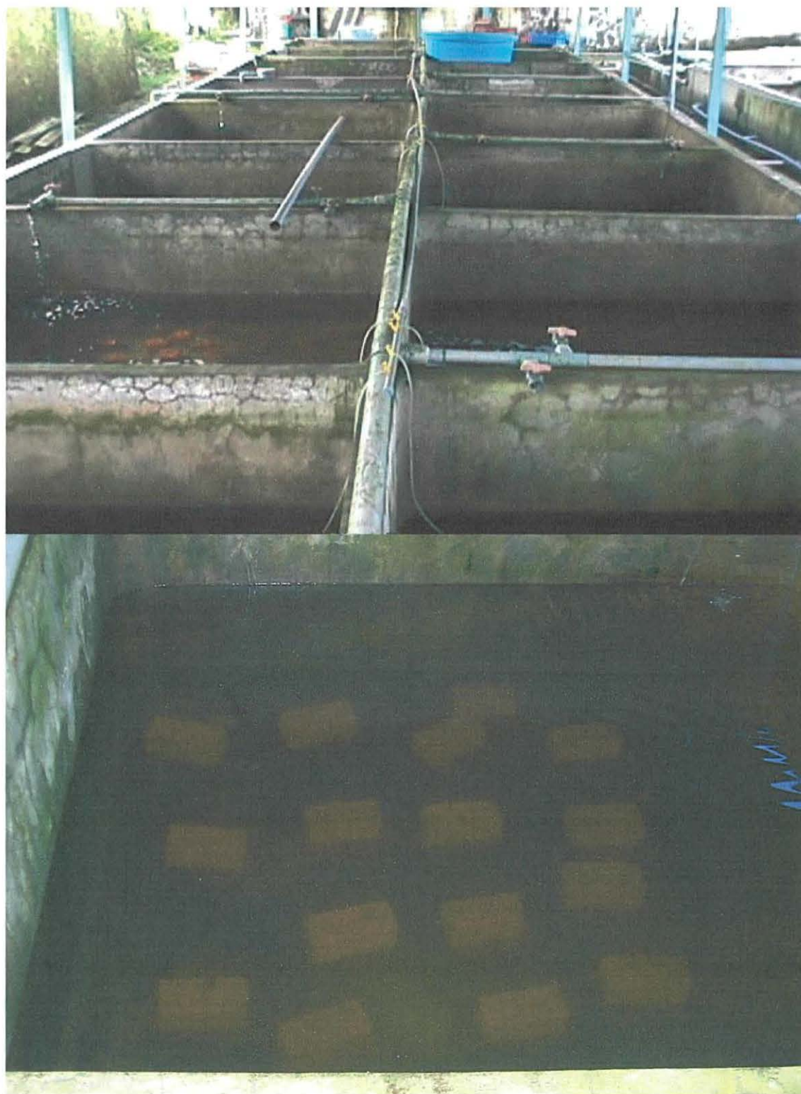
Figure 1: Tank recirculation system used for testing effect of shelter/substrate including sand vs bricks in Experiment 2.
