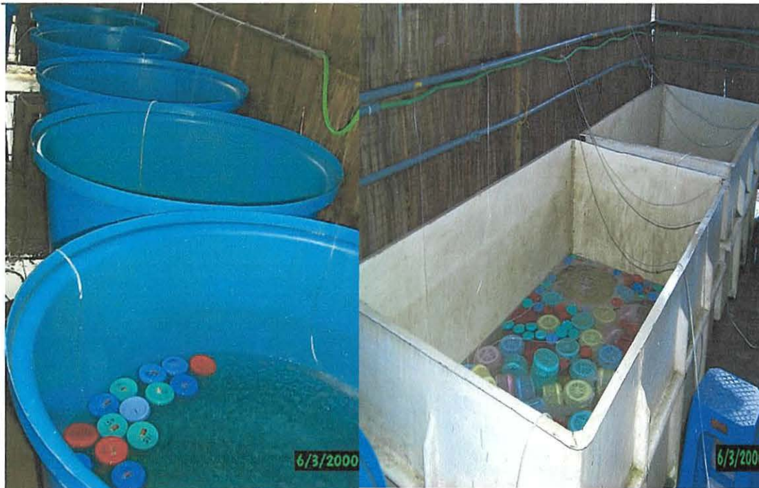
Figure 3: 500 l round and 4m 3 rectangle tanks used as a batch system for salinity experiments carried out in Vinh Chau station.
