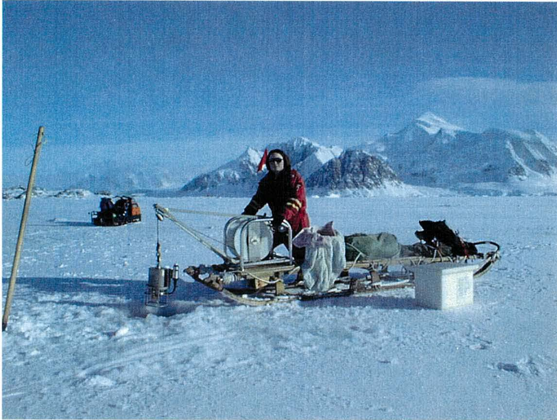
Fig. 4.2. Photograph showing water sampling through a conductivity-temperature-depth (CTD) unit cast at the Rothera Time Series (RaTS) site at 15 m depth in Ryder Bay, Adelaide Island, western Antarctic Peninsula in austral winter. The collection of water samples was carried out through a hole drilled in the consolidated pack ice. The photograph was provided courtesy of A. Clarke, British Antarctic Survey.
