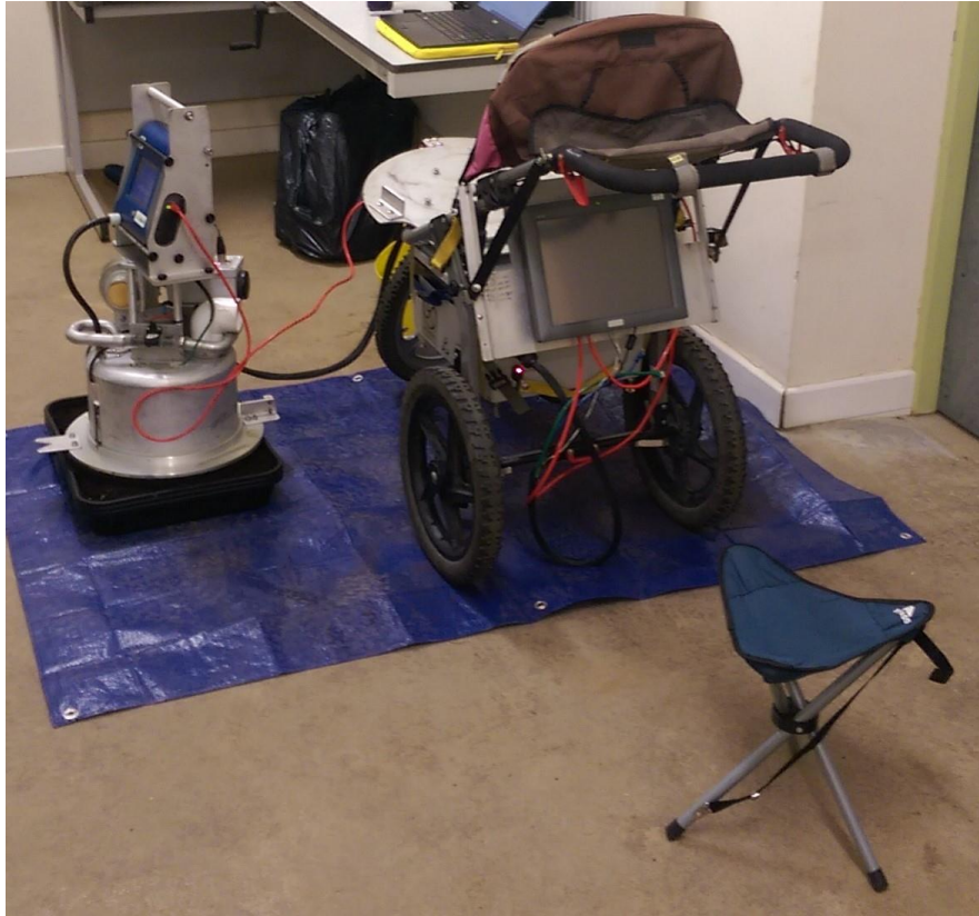
Figure 4.2. Demonstration of the experimental setup. Shows the PI-SWERL chamber in position on a prepared tray.
