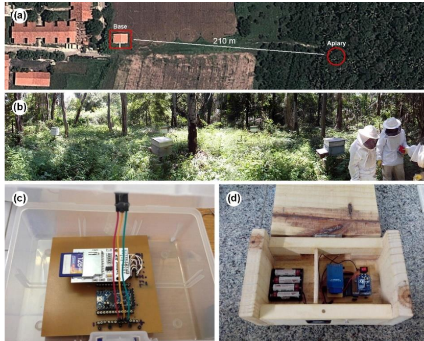
Figure 2.16 The physical setup of Kridi et al., showing (a) the distance from the observation base, (b) the environment surrounding the apiary, and (c and d) the prototype in plastic and wooden protection, respectively [118].
