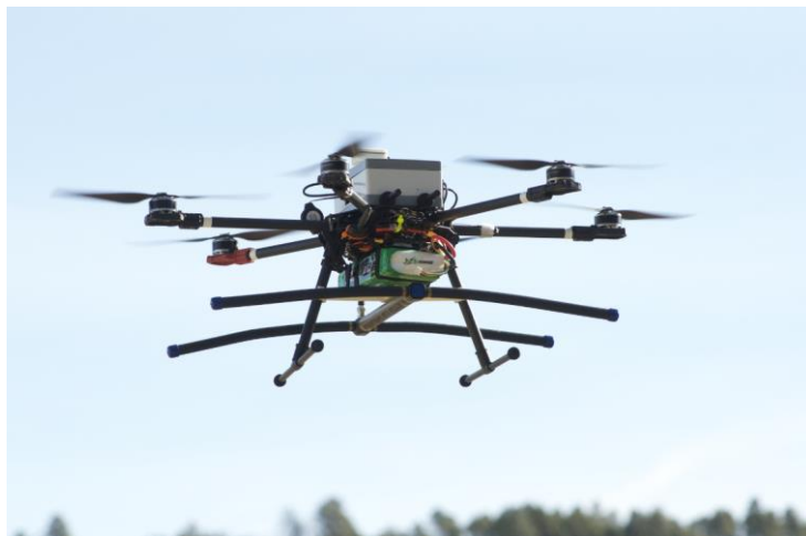
Figure 2.10 Prototype drone with antenna system [75].
