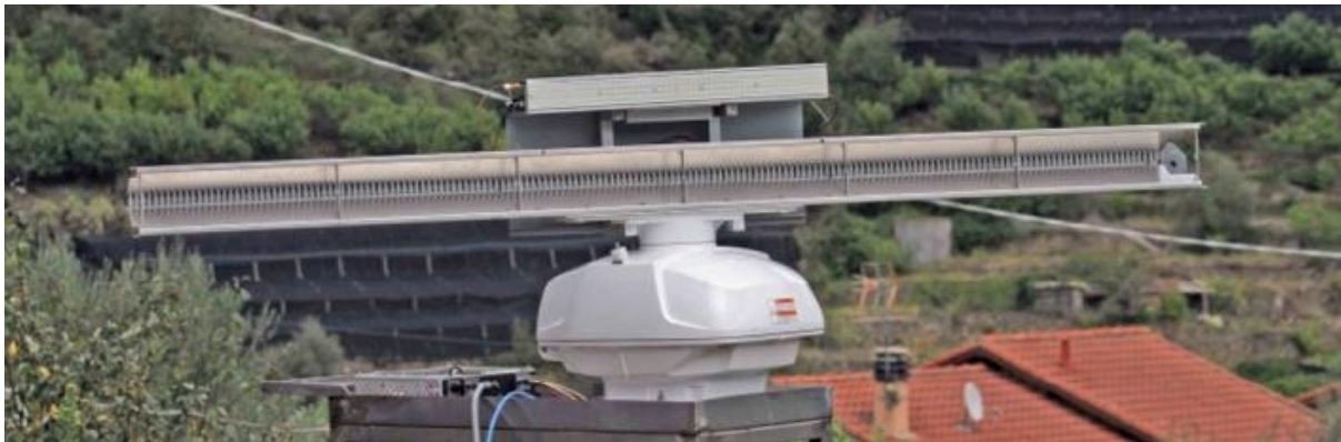
Figure 2.5 Harmonic radar for hornet tracking. The transmitting antenna is 180 cm long, while the receiving antenna, on top, is 50 cm long [46].
