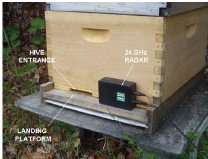
Figure 2.14 24 GHz Doppler radar mounted at the entrance to a beehive [109].
