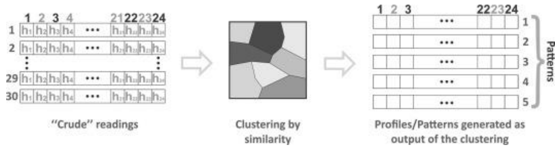
Figure 2.15 Conceptual creation of thermal patterns from raw data. These were the source patterns that new measurements were compared with to determine deviancy [118].
