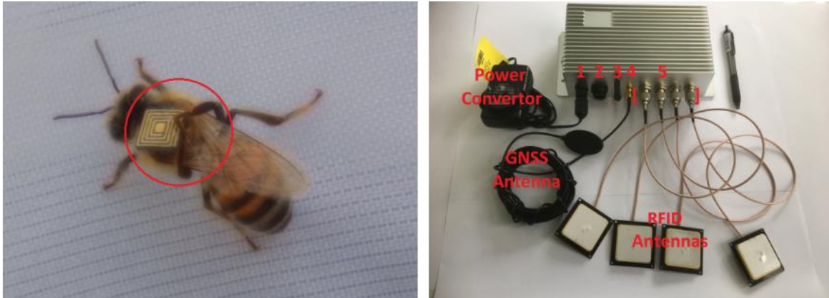
Figure 2.6 Example of a bee disturbed by the RFID tags. Aluminium housing (18.5 cm × 10.5 cm × 5.5 cm) and peripherals. (1) 4-pin power inlet; (2) micro-USB port; (3) Wi-Fi antenna; (4) GNSS antenna, and (5) RFID antennas and ports [55].
