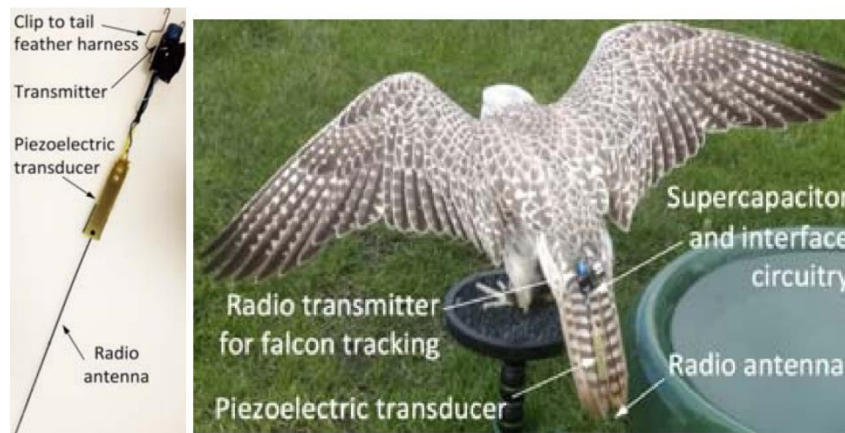
Figure 2.11 Piezoelectric energy harvester used to track a hawk over large distances [83].
