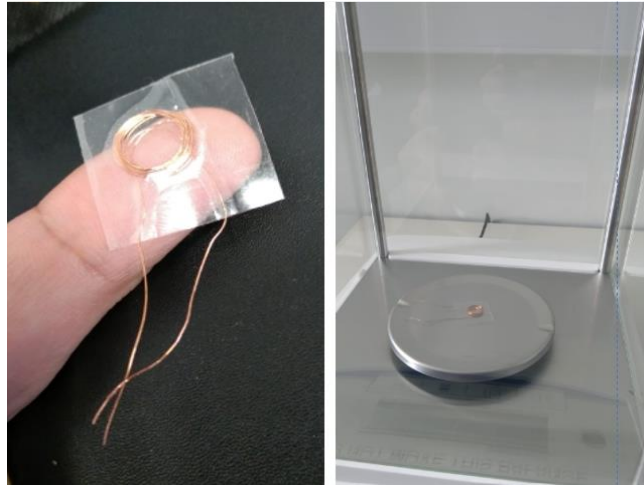
Figure 2 Primary coil for the testing of inductor antennas.
