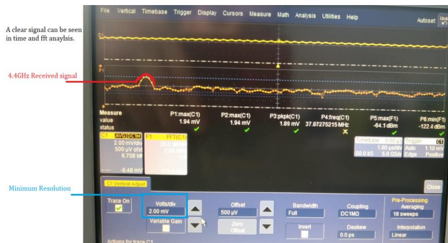
Figure 15 An advanced oscilloscope was used to sweep the frequency to detect the slightest of signal induced in the secondary coil
