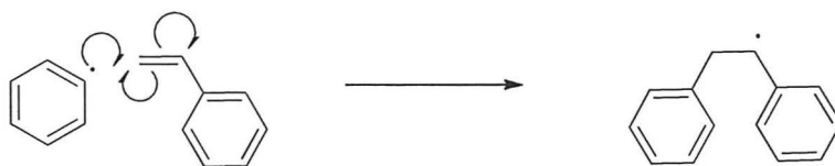
Figure 19: Phenyl initiator from benzoyl peroxide (BPO) attacks a styrene molecule to start the polymer chain
