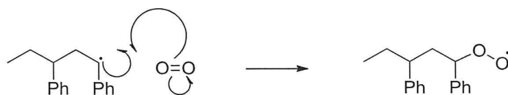
Figure 22: Termination of Polystyrene by reaction with radical initiator.
