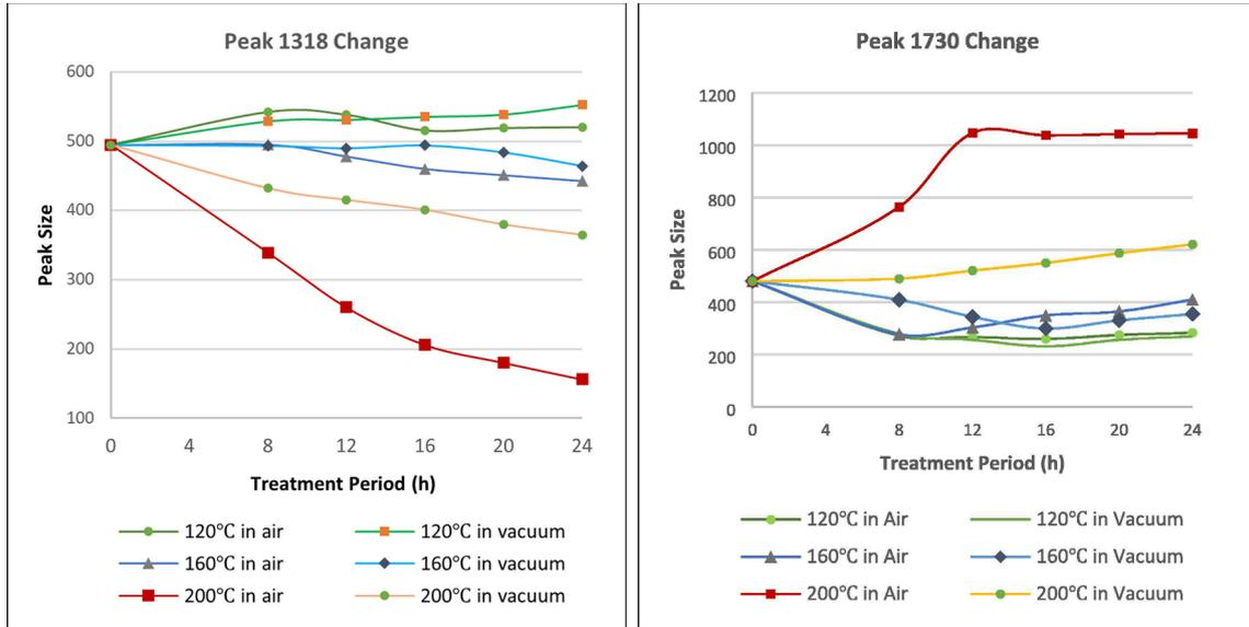
**Fig. 8.** FTIR Peak Size Changes of Peak 1318 cm<sup>-1</sup> and 1730 cm<sup>-1</sup> during Thermal Treatment.
