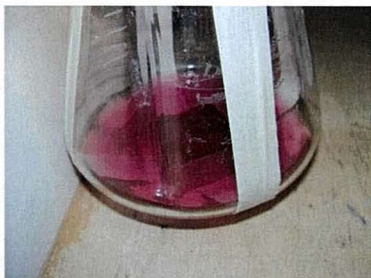
A. The colloid is placed against a 1.3 T magnet and the pH adjusted to 7
