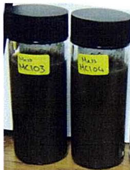
Figure 4.1.2. SPION produced from the Massart method. 150 Left image, SPION in 1 M TMAOH and right image, SPION after stirring with 2 M perchloric acid, isolating by centrifuging and peptising with deionised water.
