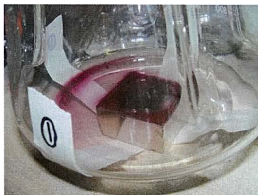
B. Particles migrate to the magnets surface, those furthest taking longer to travel
