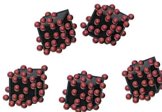
D. Illustration of Au seeded Fe_3O_4 after magnetic recovery from seeding solution
