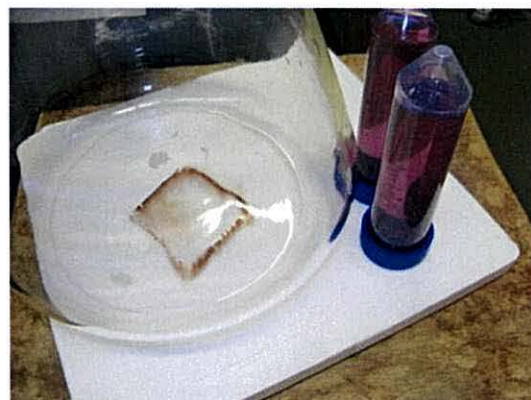
D. The bare \gamma -Fe 2 O 3 particles flocculate without the stabilising Au surface coating
