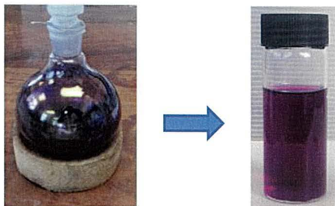
Figure 4.37. Photographs of (a) solid ( 38 ) after drying under high vacuum, (b) a solution of ( 38 ) 1 \times 10^{-4} M dissolved in MeOH.
