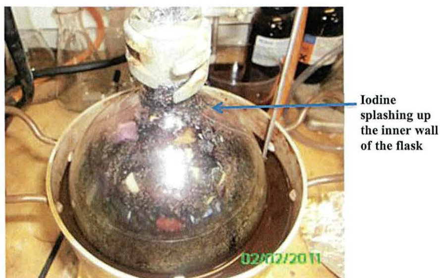
Figure 5.19. Iodine splashing on the inner wall flask during synthesis of 4,5-diiodophthalimide ( 17 ) reaction using fuming sulfuric acid.
