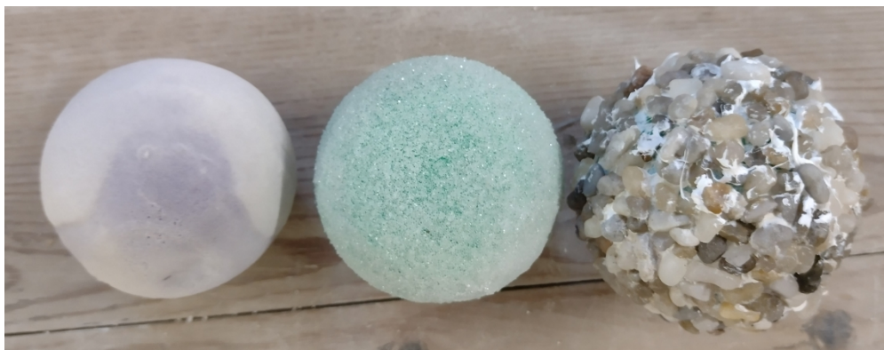
FIGURE 4 Examples of spherical tools with sediment armour used in the experiments. The diameter of each sphere is 0.05 m. From left to right: tool with silt to very fine sand armour, tool with coarse sand armour and tool with gravel (pebble) armour.
