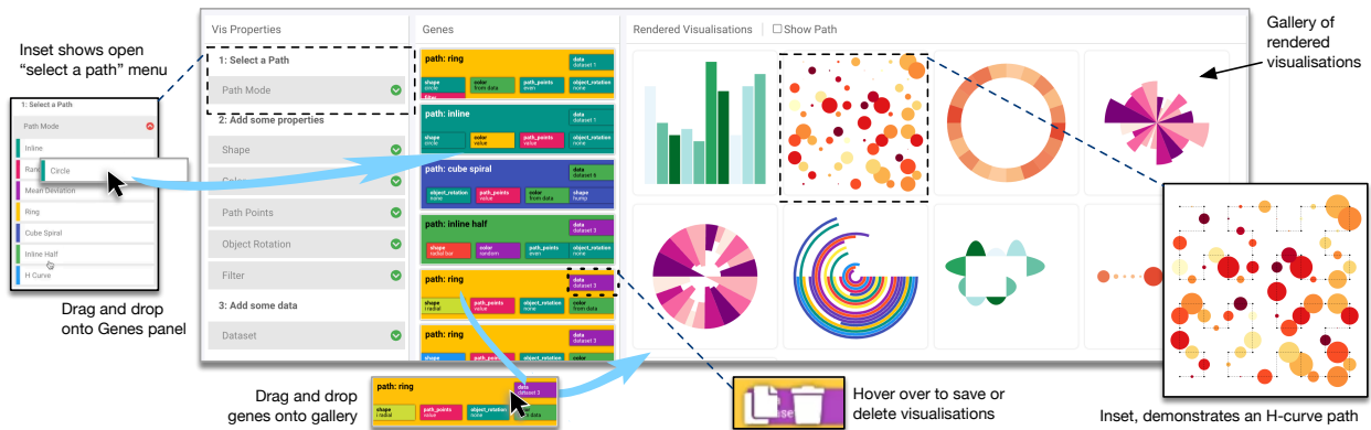
Fig. 1: The Genii visualisation designer that demonstrates our flowpath model. Individuals define their own path or choose predefined flowpaths (left panel), drag and drop the visualisation properties into the gene panel (middle), which are rendered onto the gallery (right). Users can either create a new gene which adds a new image to the gallery, or edit parameters (through drag and drop) to adapt current visualisations. Crafted visualisations can be exported and used in other applications.
