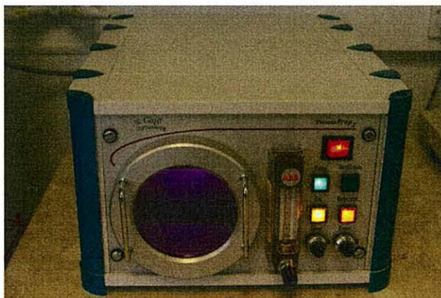
Figure 2.25: The Gala Instrumente Plasma Prep II in operation, showing the glowing nitrogen plasma inside the chamber.
