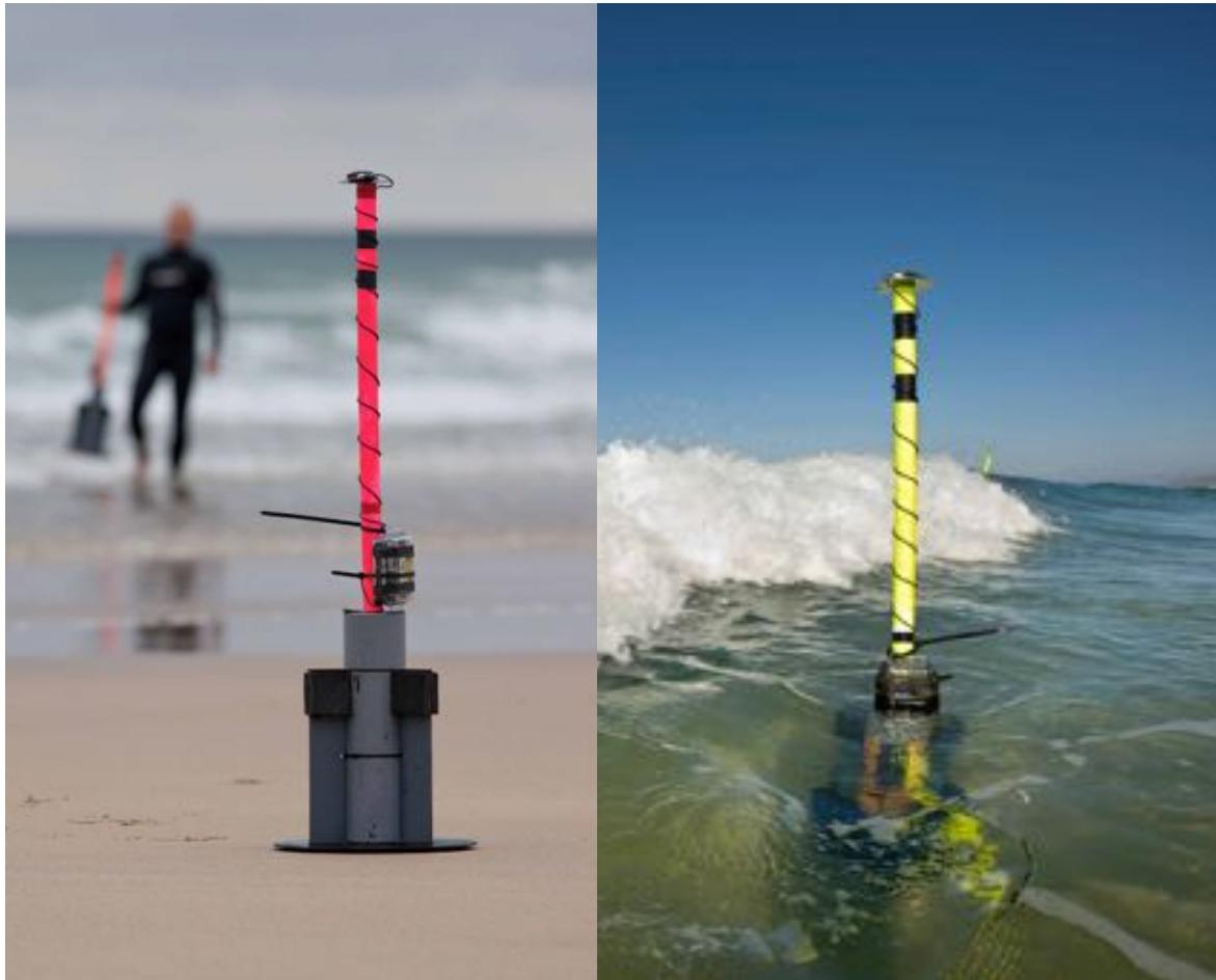
**Figure 4** – GPS drifter unit. Drifter body is constructed of a buoyant chamber with a damping plate and fins to reduce surfing. When floating, only the coloured mast is visible on top of which is the GPS antenna attached to a ground plane. Steel ballast plate ensures quick righting and minimum signal loss due to waves. GPS unit is secured in a waterproof box fixed the mast.
